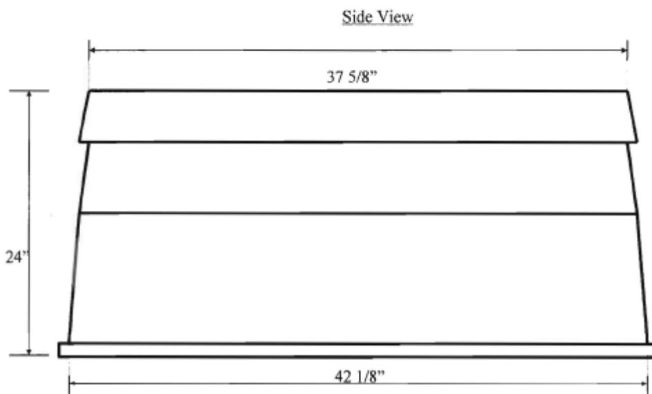
30" x 48" x 36" Fiberglass Composite Meter box
