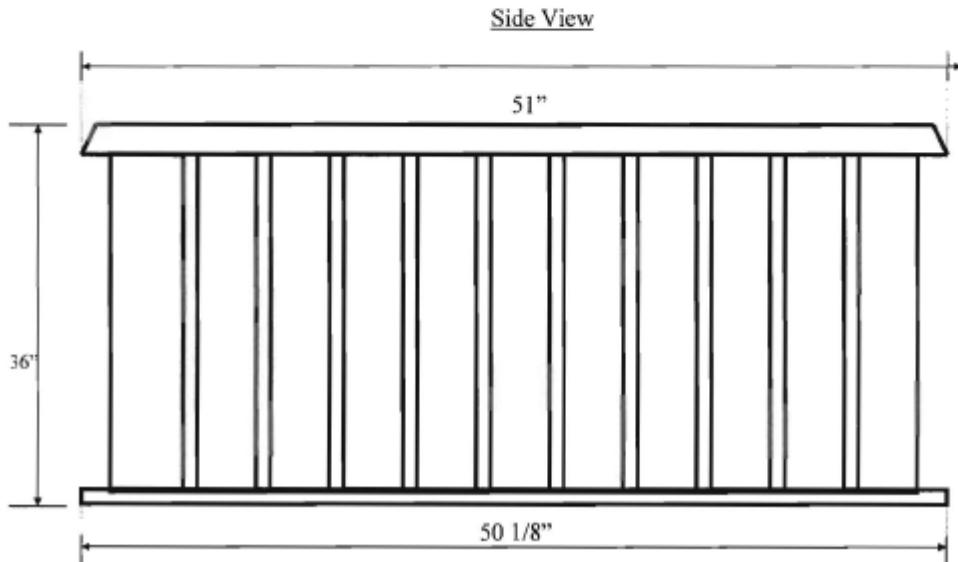
36" x 60" x 36" Fiberglass Composite Meter box
